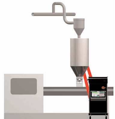
Dryer on the floor; hopper on the throat.
