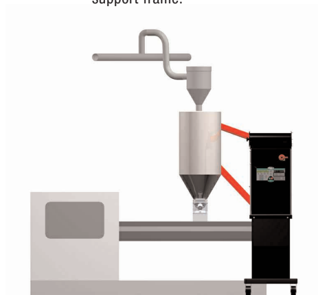
Dryer on a floor stand; hopper on the throat.
